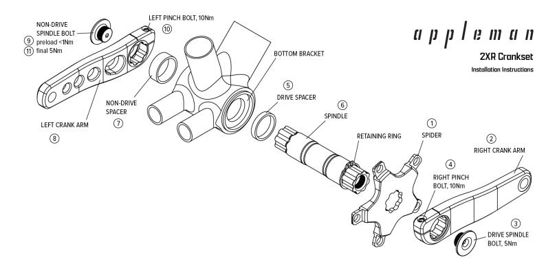
NOTE: Grease all surfaces that touch each other during installation or use. Grease entire spindle surface including lobes and bearing surfaces Grease threads, under bolt heads, all metal mating surfaces etc... Proper greasing will ensure durability and maintainability of the cranks. BONUS: pinch bolts, retaining ring, spindle bolt threads have factory grease applied.
