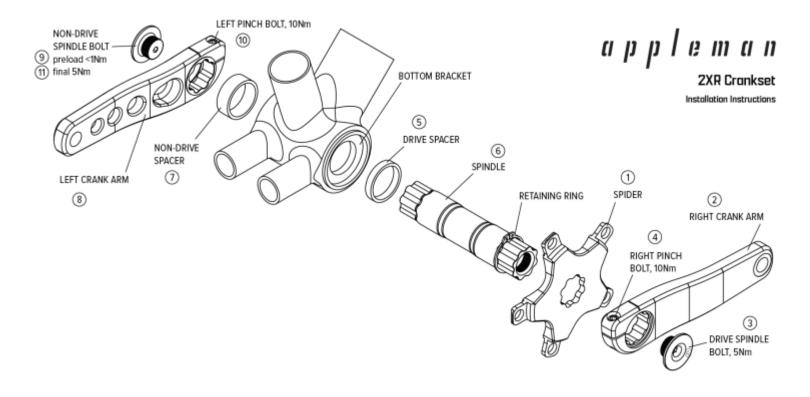
NOTE: Grease all surfaces that touch each other during installation or use. Spindle lobes, bearing surfaces, threads, under bolt heads etc... Proper greasing will ensure durability and maintainability of the cranks. BONUS: pinch bolts, retaining ring, spindle bolt threads have factory grease applied.
